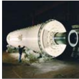
Ball Mill for Lime Plant installation
