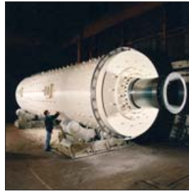
Ball Mill for Lime Plant installation
